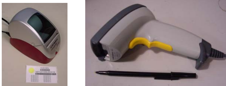
Figure 6: Dymo Labelwriter Turbo 330 printer and LS4000i handheld barcode reader
