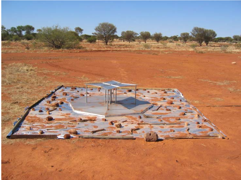
Figure 5. EDGES in “absolute sky noise” mode with temporary extended ground plane.
