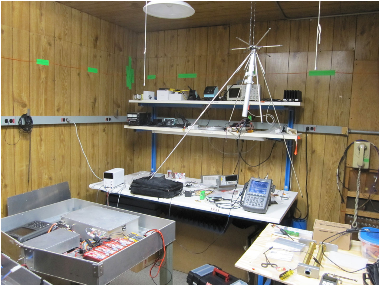
Figure 1. Set-up for tests of emissions from EDGES-3 electronics.
