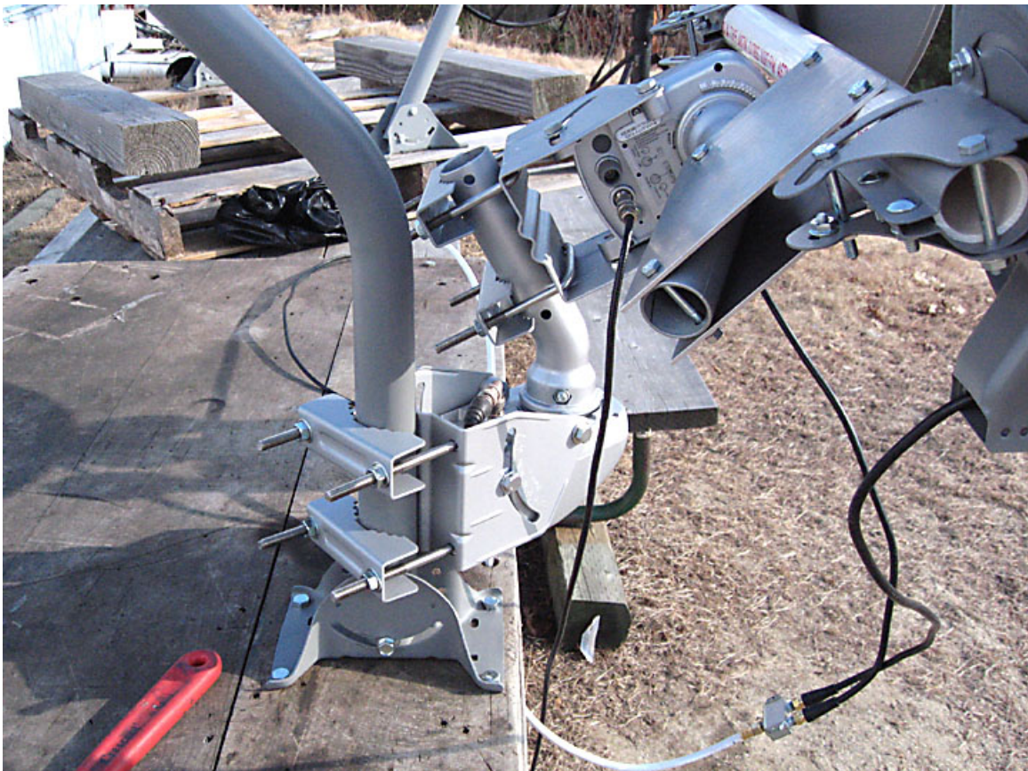
Figure 2. Azimuth/elevation mount using 2 DiSeQC SG2100 motors
