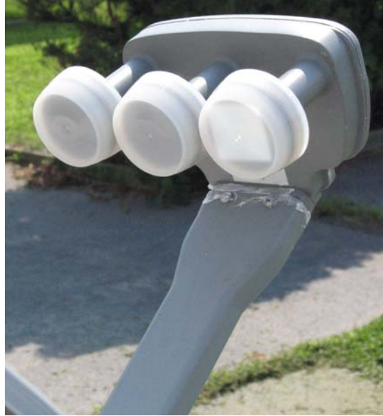
Figure 3.1.2.1: Triple feed LNB is active
