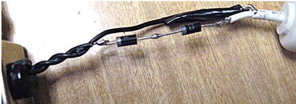
Figure 3.3.3: Diode drop for DC Power Injector
