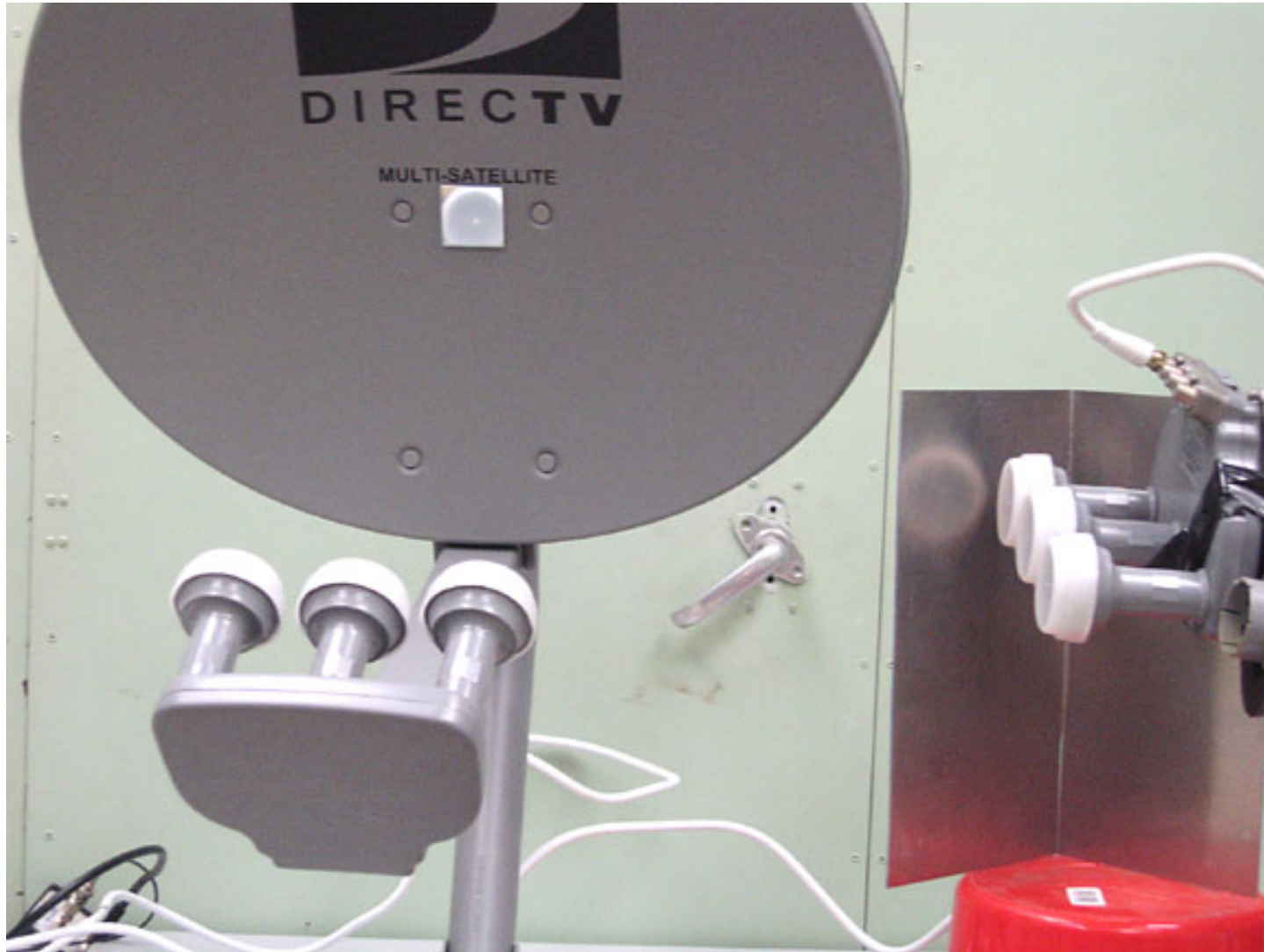
Figure 5. 2-element interferometer using DirecTV dish the view is from the CFL signal source. Note: the optical reflections of the active feed used as an initial alignment guide and LNBF as a “reference” antenna.
