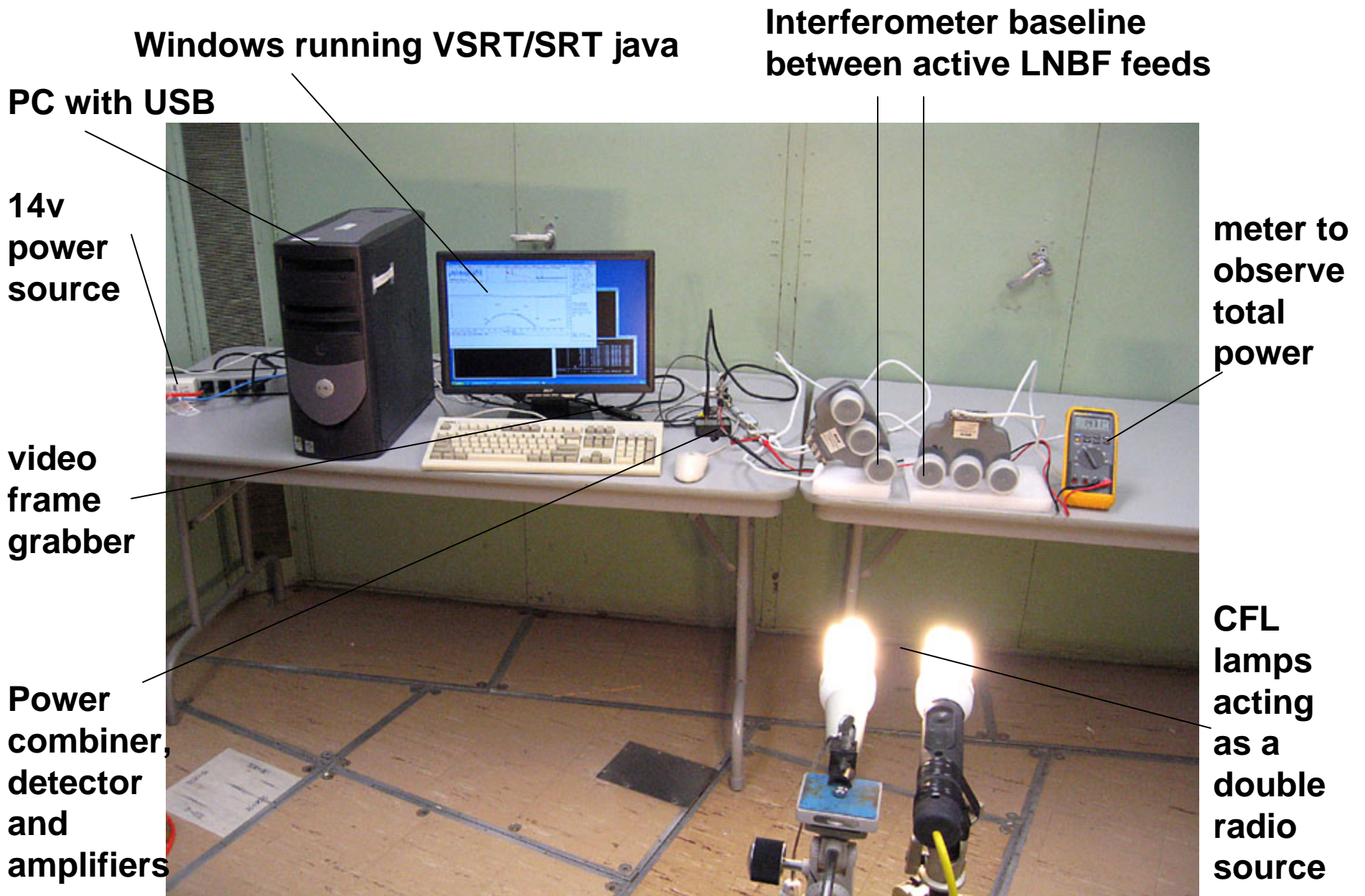
Simple laboratory setup to demonstrate the principles of radio interferometry
