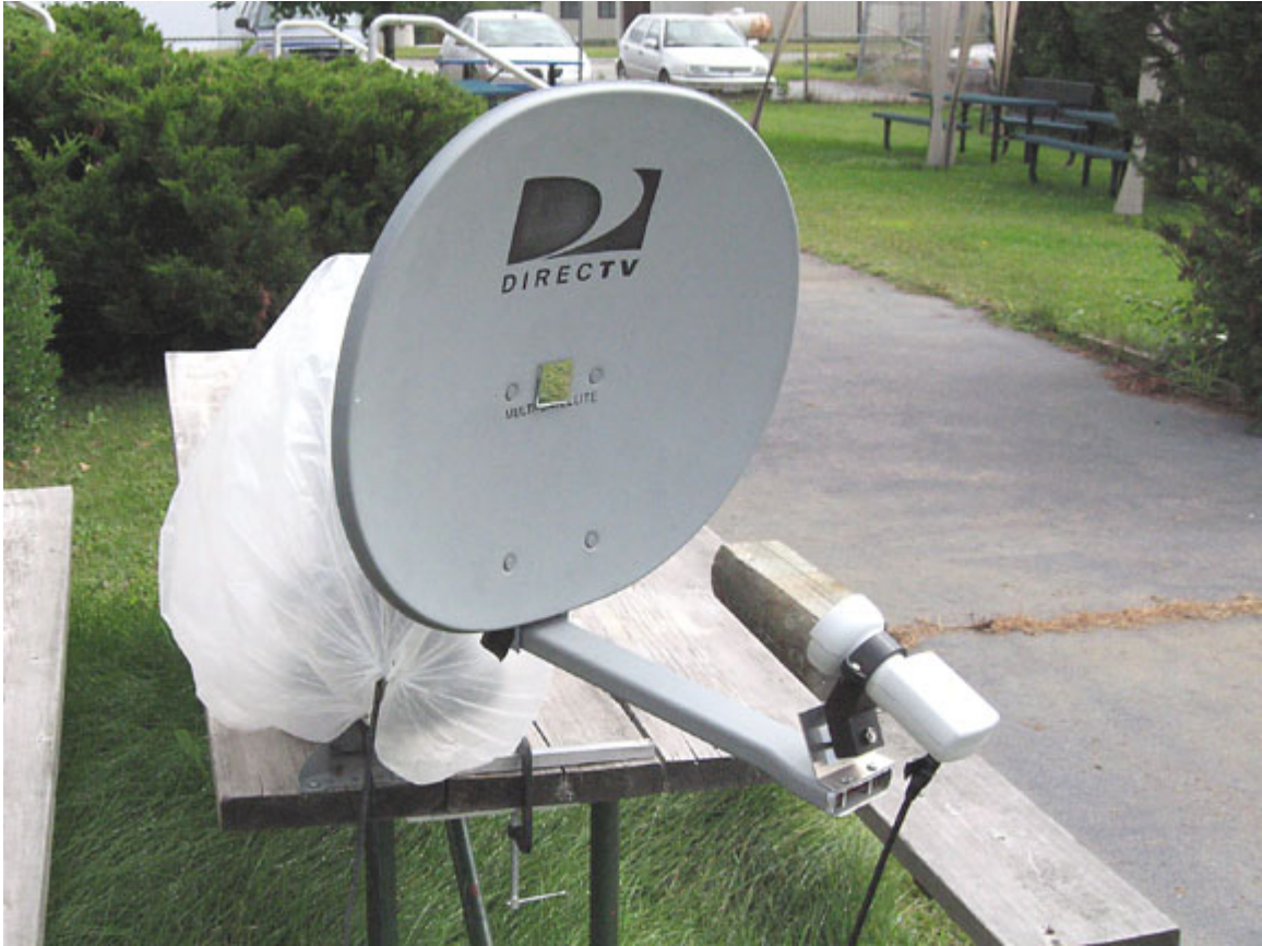
Figure 3 VSRT antenna and LNB set-up to observe the 11 GHz ozone line in the Mesosphere.
