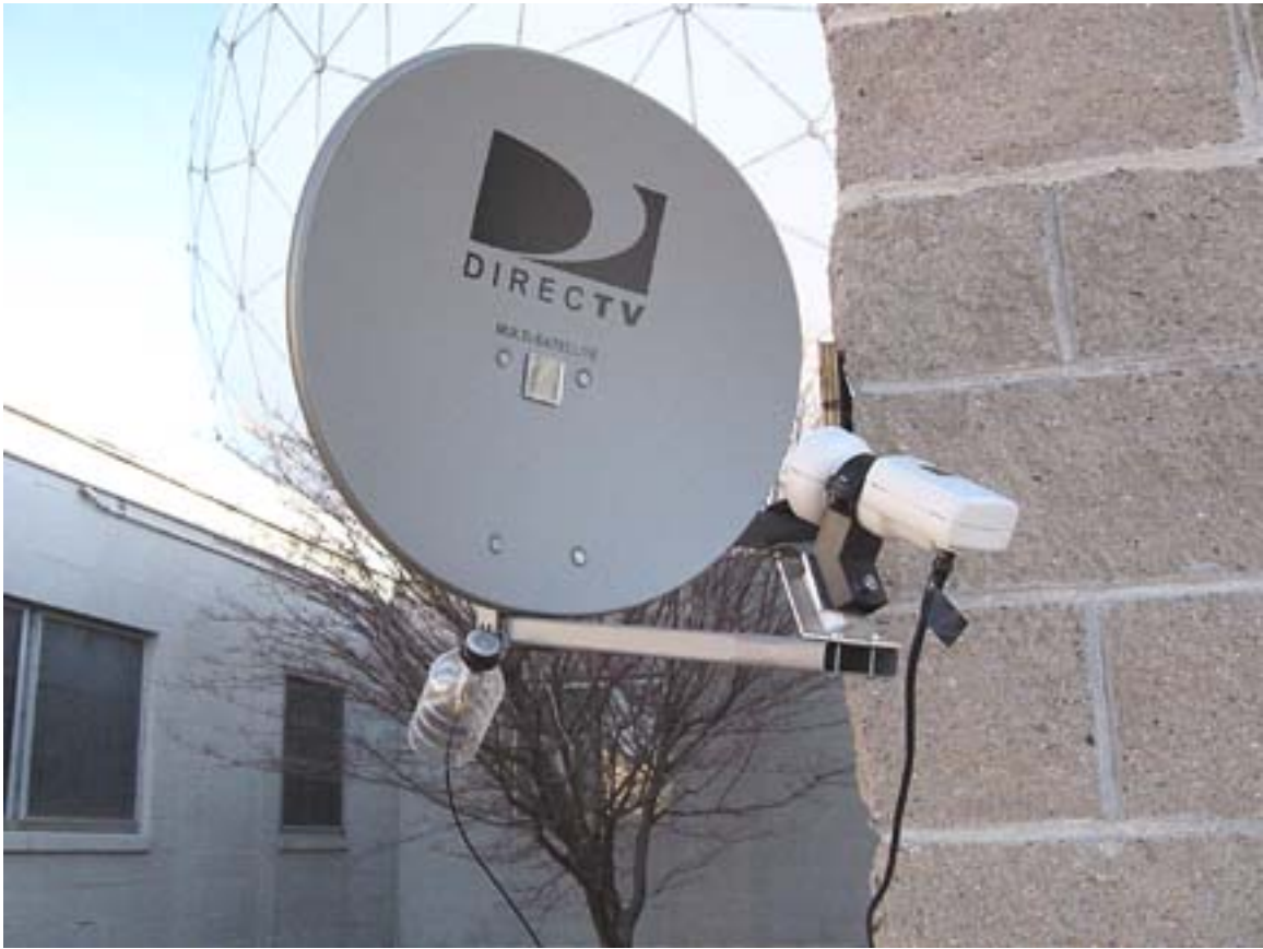
Figure 2. Fixed 18" dish set to observe at 8 degrees elevation at about 180° azimuth at the Haystack Observatory. The dish and LNB assembly weighs about 10 lbs.
