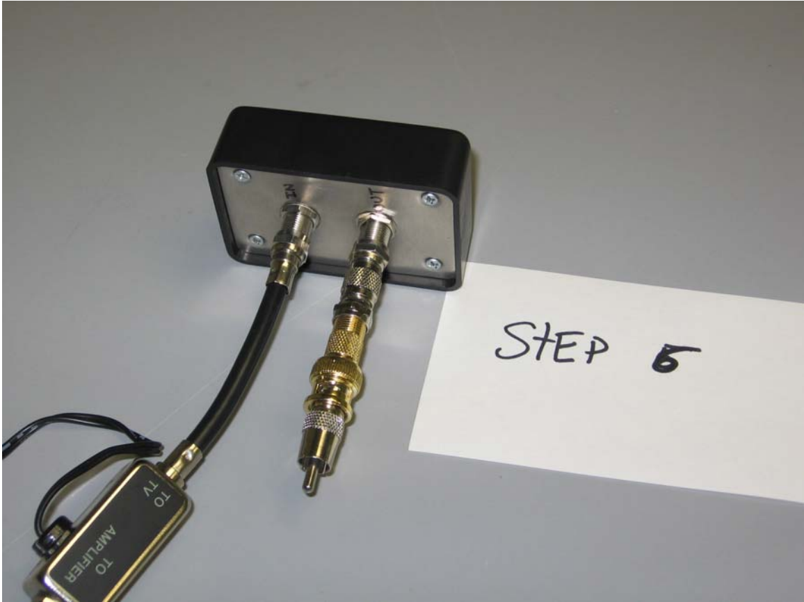
Figure 11. Step 6: Attach the detector. Details of the inside of the box are shown in Figure 4. Also attach the necessary connectors.
