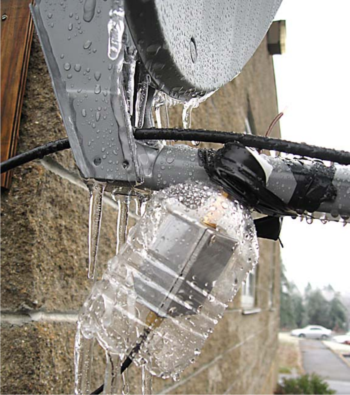
Figure 5a. When correctly assembled the end of the calibrator probe should be at an angle of 45° degrees.
