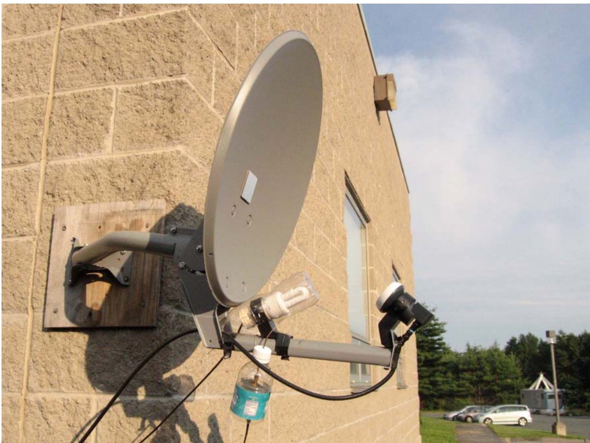
Figure 1. Ozone spectrometer at Haystack with CFL lamp for calibration tests.
