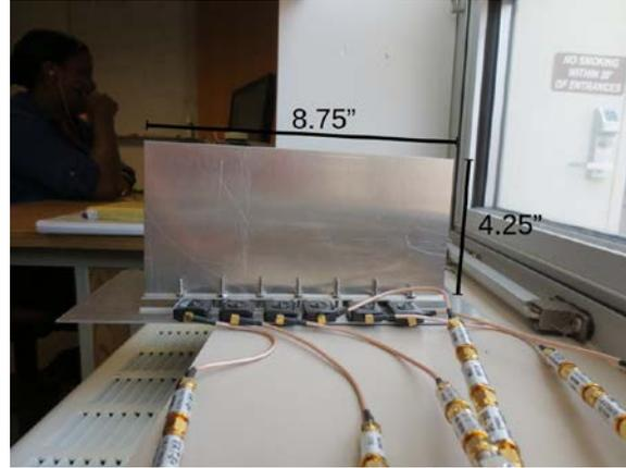
Since the current drawn by the Hub was 840 mA supplied from a 12 V source about 10 W was dissipated in the circuit. Assuming that the majority of the power dissipated was in the dongles, we can assume that about 10 W will need to be dissipated by the heat sink. To find the power dissipated due to radiative transfer we can use the equation.
