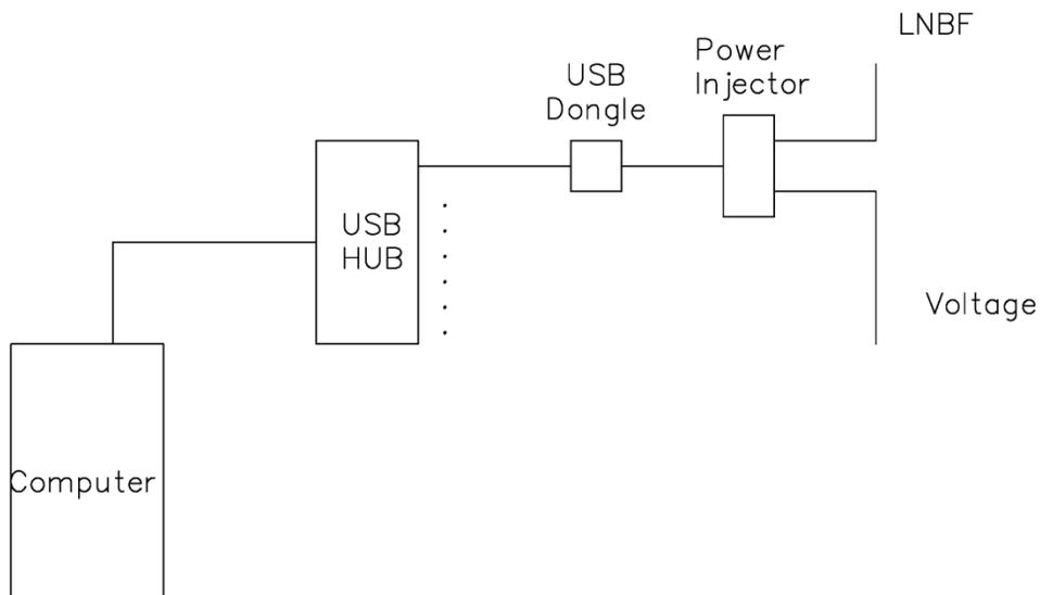
However under this configuration, the USB digital TV tuner RTL-SDR dongles were overheating to a temperature of 55°C as measured at the RF input connector. At a temperature around 55°C and above the local oscillator synthesizer fails.
