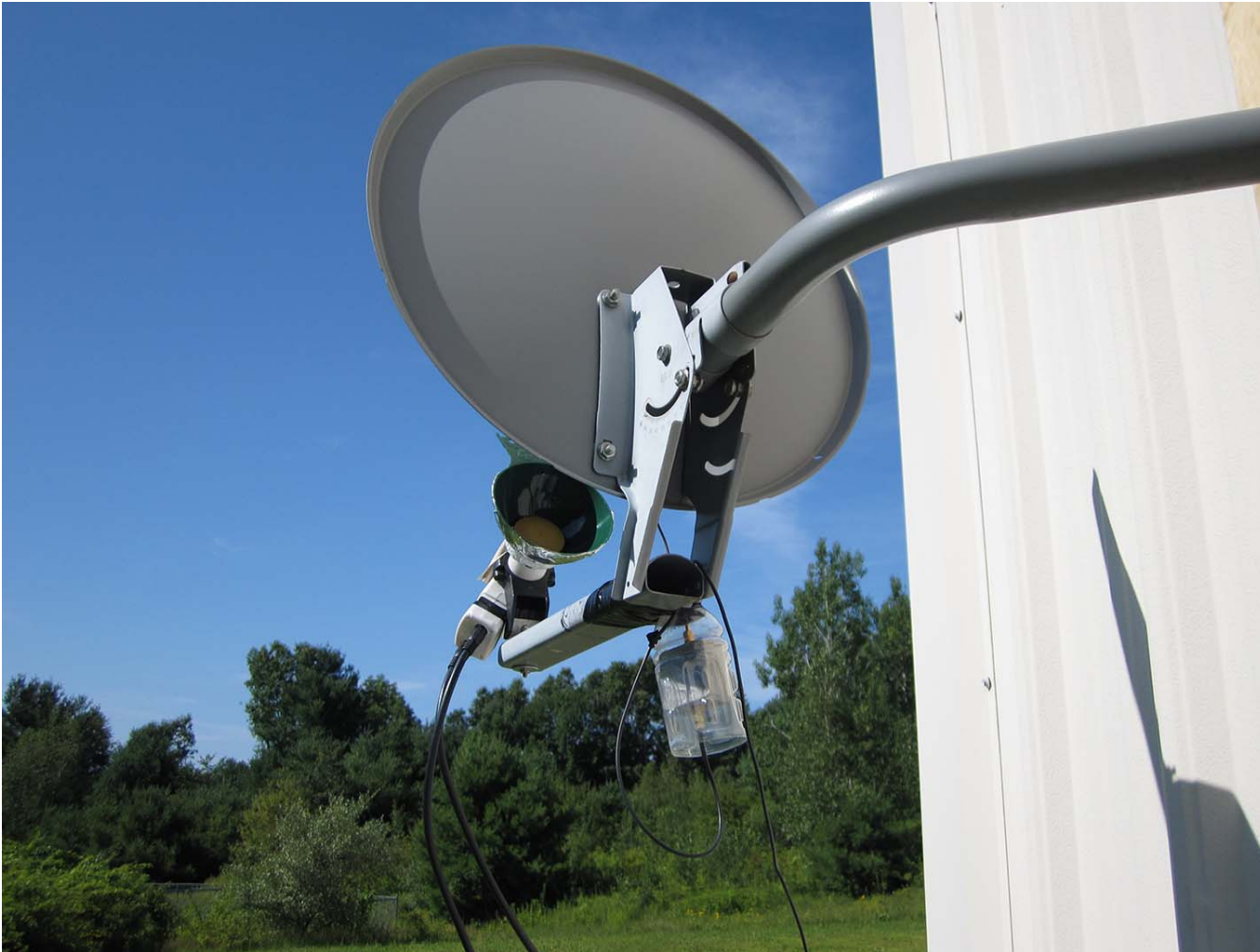
Figure 4. Tests of a shield on LNBF
