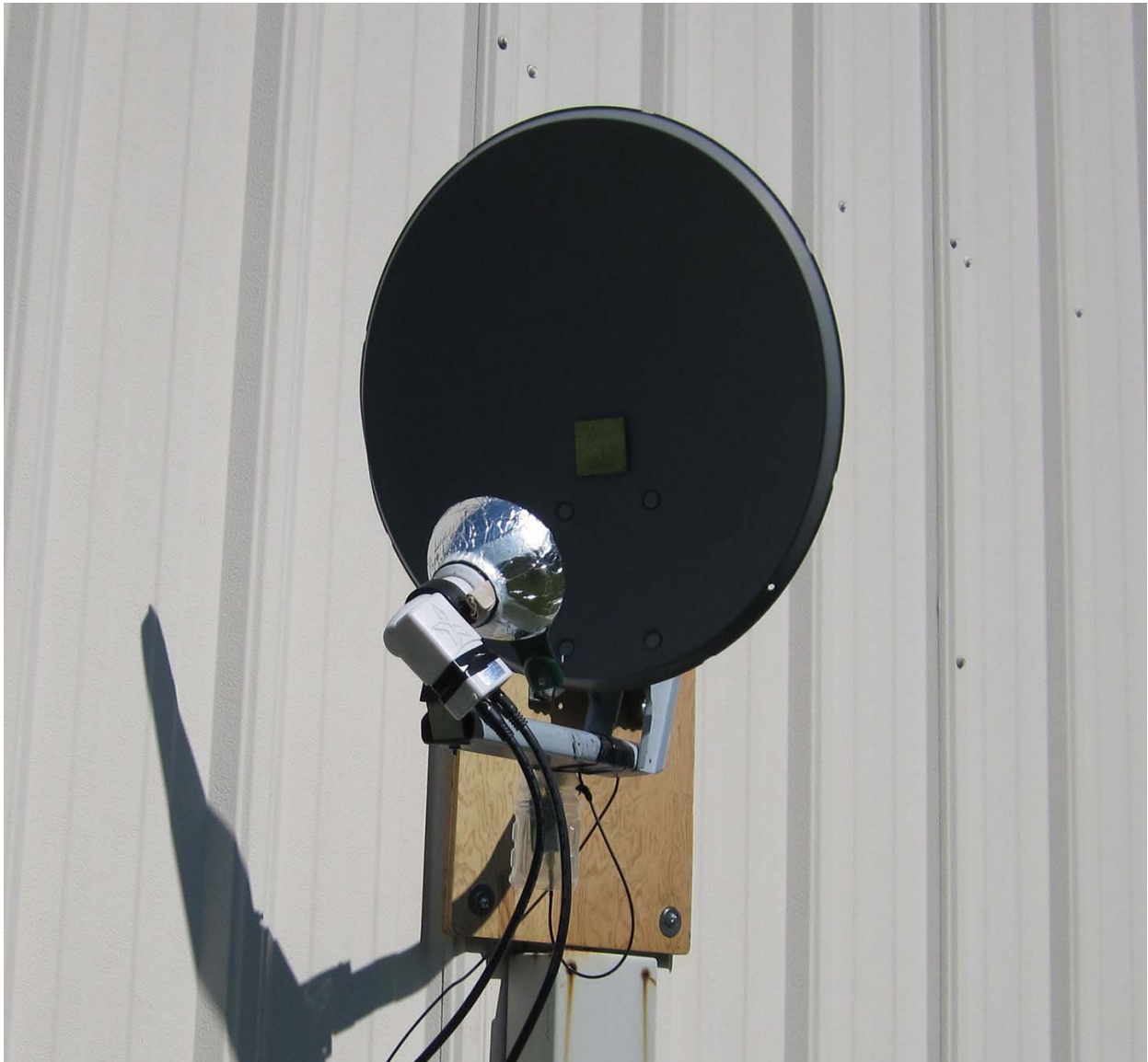
Figure 5. LNB shown with “test” shield on LNB.
