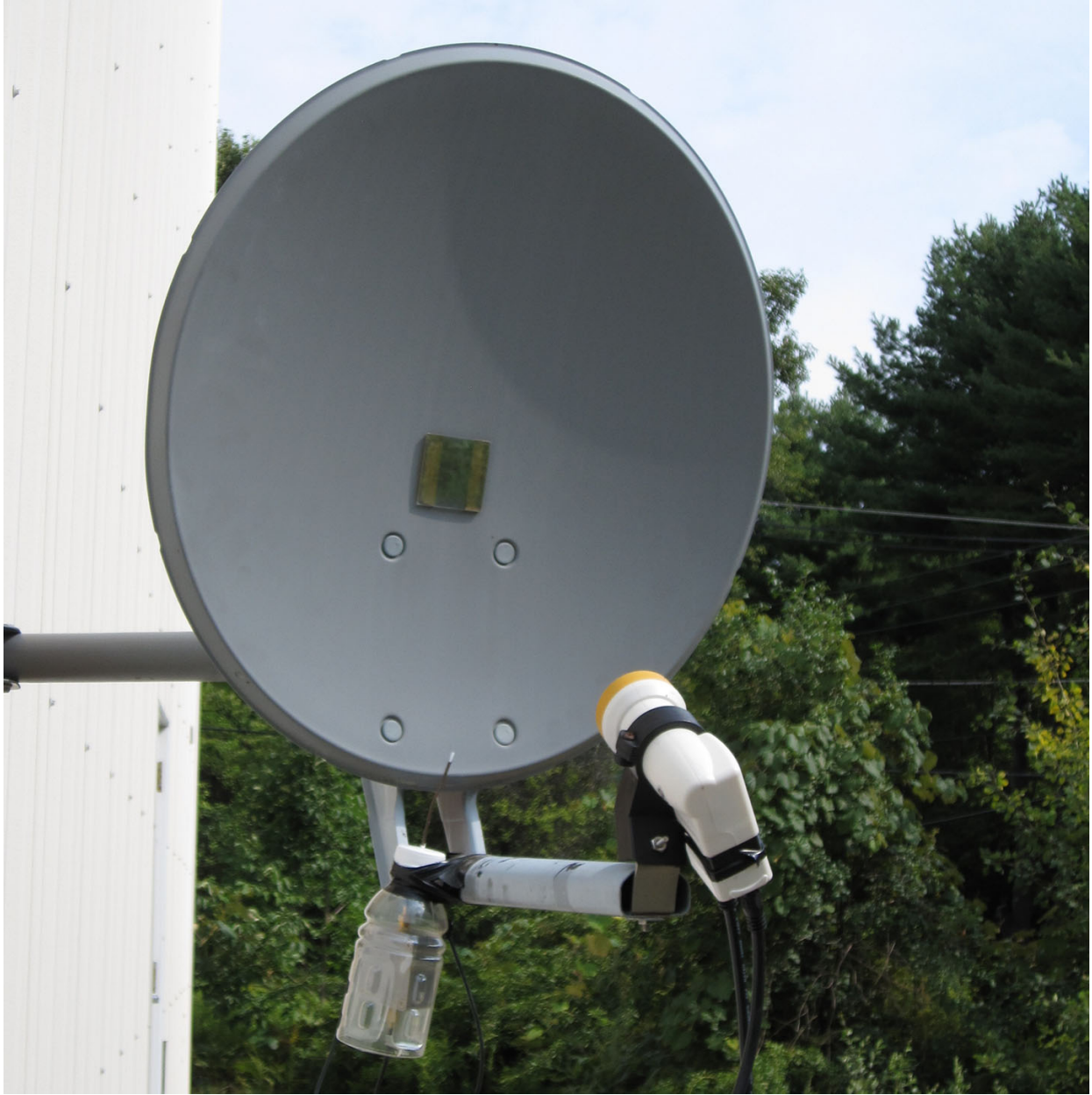
Figure 6. Close-up view of antenna, frequency calibrator and LNBF mounting bracket.
