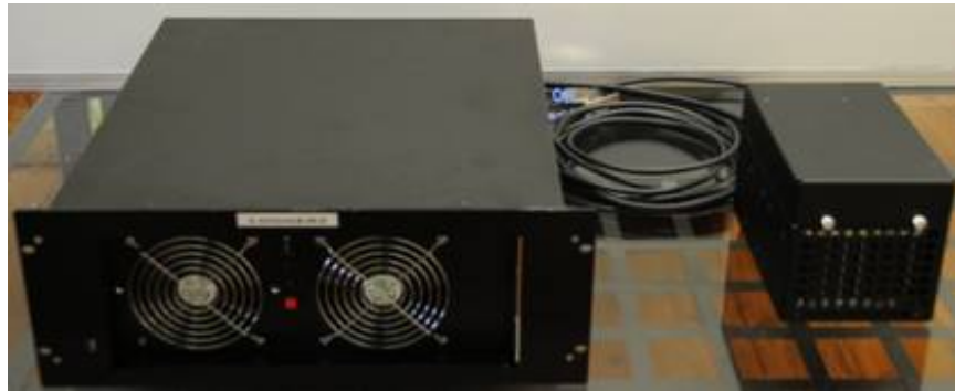
Figure 1: Front view of Mark 6 controller with disk module
