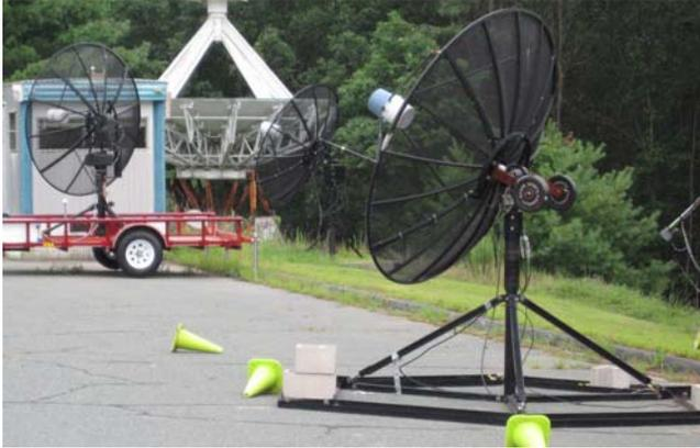
Figure 1: The SRTs used in the 3-element interferometer. In the foreground is SRT3. The left-most antenna on the red trailer is SRT1 and the remaining antenna is SRT2.
