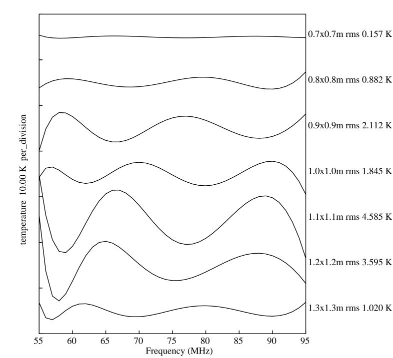
Figure 3. Residuals for loss as in figure 1 for square ground planes from 0.7x0.7m to 1.3x1.3m.
