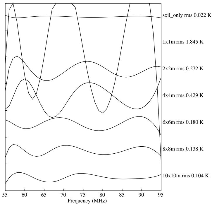
Figure 1. Residuals to 5-term fit to spectrum with loss calculated from beam fraction below the horizon for uniform soil with dielectric 3.5 and zero conductivity.
