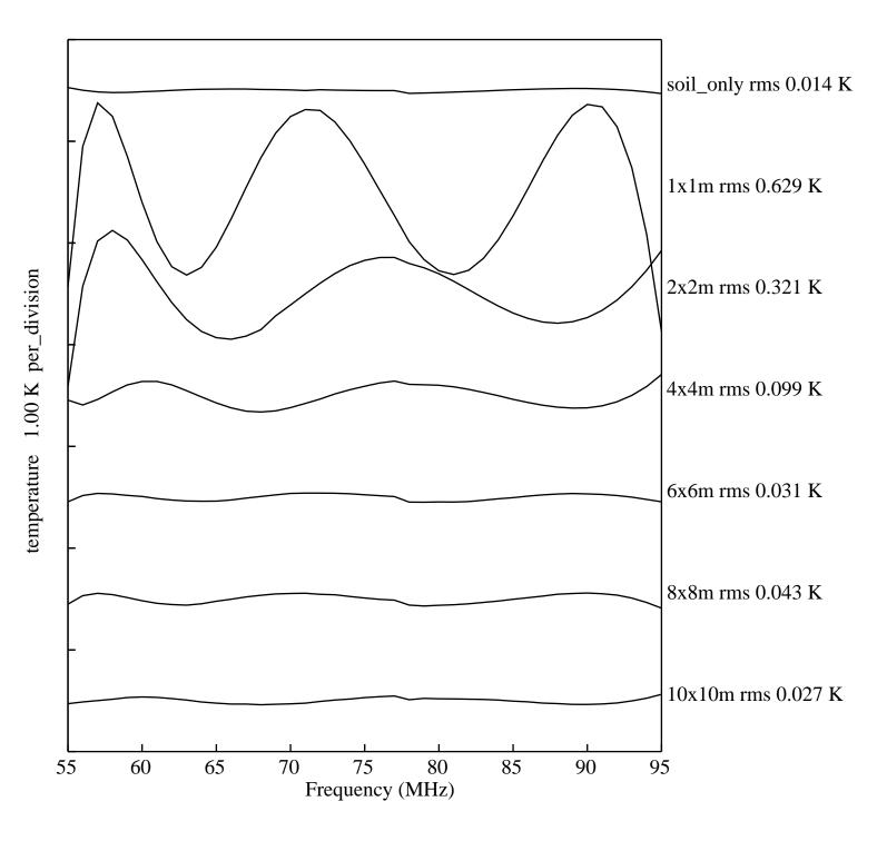
Figure 2. Residuals with loss calculated from beam fraction difference from unity when integrated over the gain above horizon using the GF method with soil dielectric 3.5 and conductivity 2e-3.
