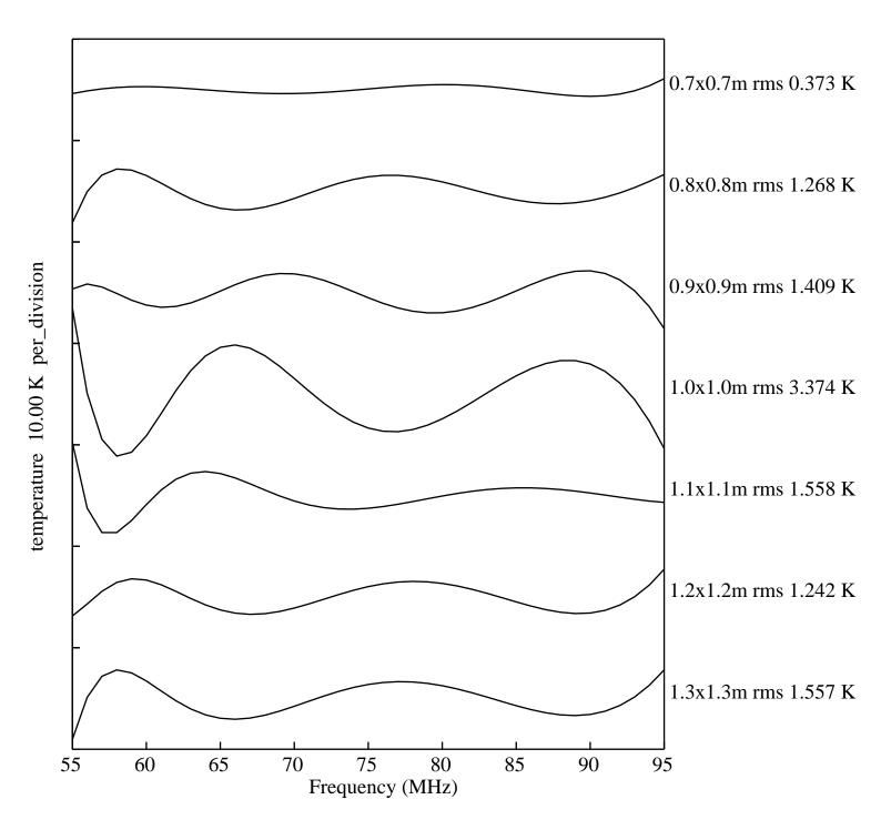
Figure 4. Residuals for loss as in figure 3 with a change in dielectric from 3.5 to 4.5.
