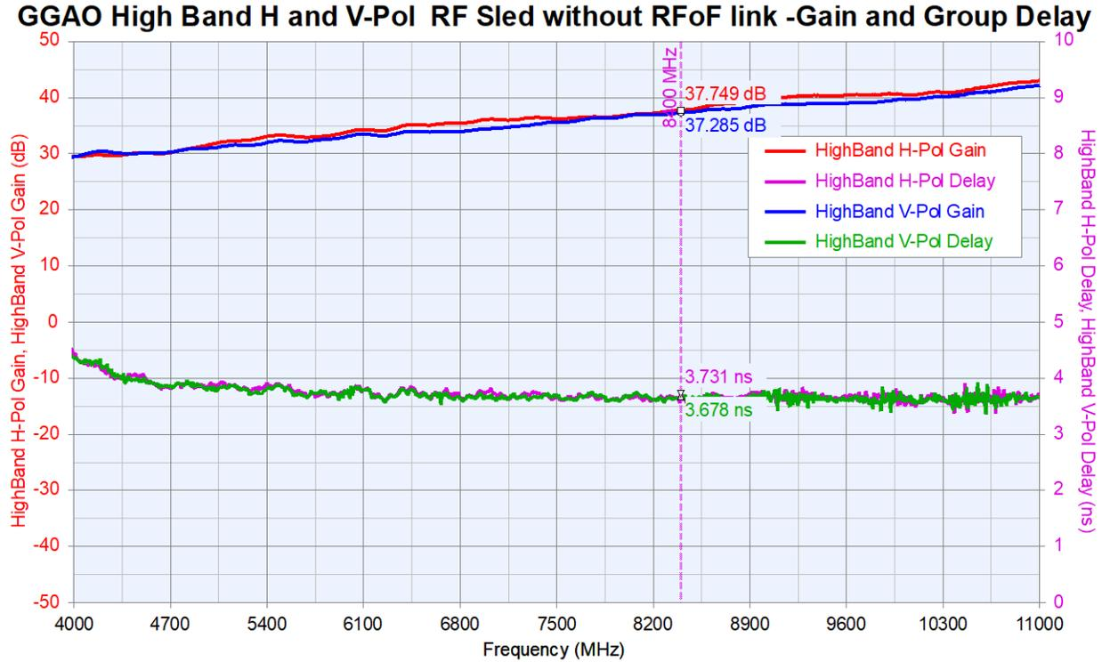
**Figure 8:** Response of the H- and V-polarization high-band filters, amplifiers, and equalizers in the RF sled.
