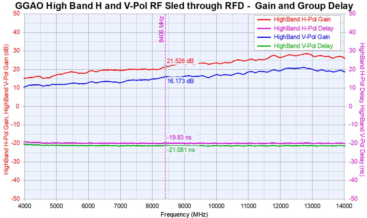
**Figure 10:** Response of the high-band H- and V-polarization post-dewar through the RF Distributor.
