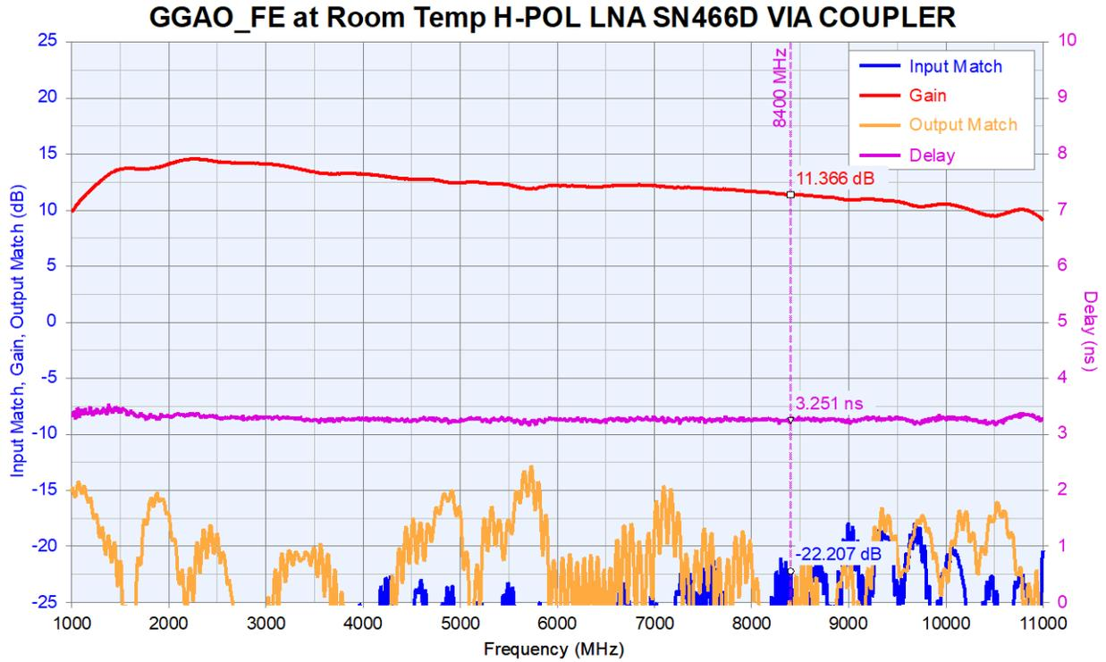
Figure 2: Measured frontend (left axis) coupled gain, input/output match, and (right axis) group delay at room temperature for the H-polarization channel.
