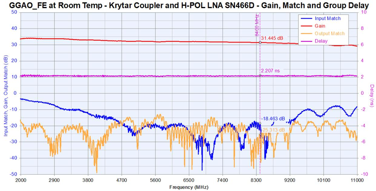
**Figure 6:** Measured frontend (left axis) straight-through gain, input/output match, and (right axis) group delay at room temperature for the H-polarization channel.
