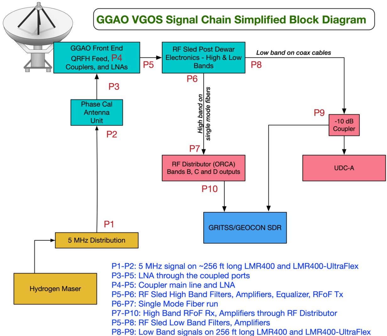
**Figure 1:** Simplified block diagram of the VGOS signal chain at GGAO.
