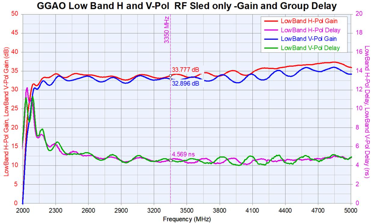
Figure 11: Response of the low-band H- and V-polarization on the RF sled.
