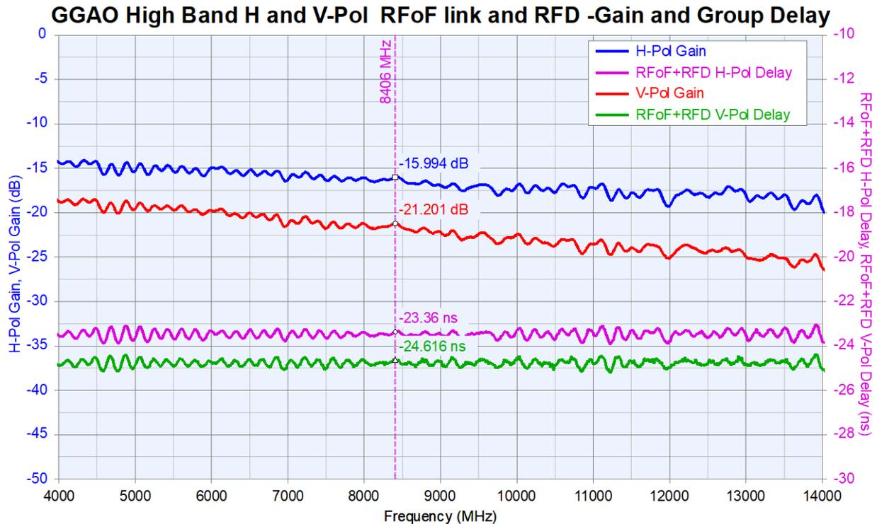
**Figure 9:** Response of the H- and V-polarization RF-over-Fiber links, amplifiers, and power dividers in the RF distributor.
