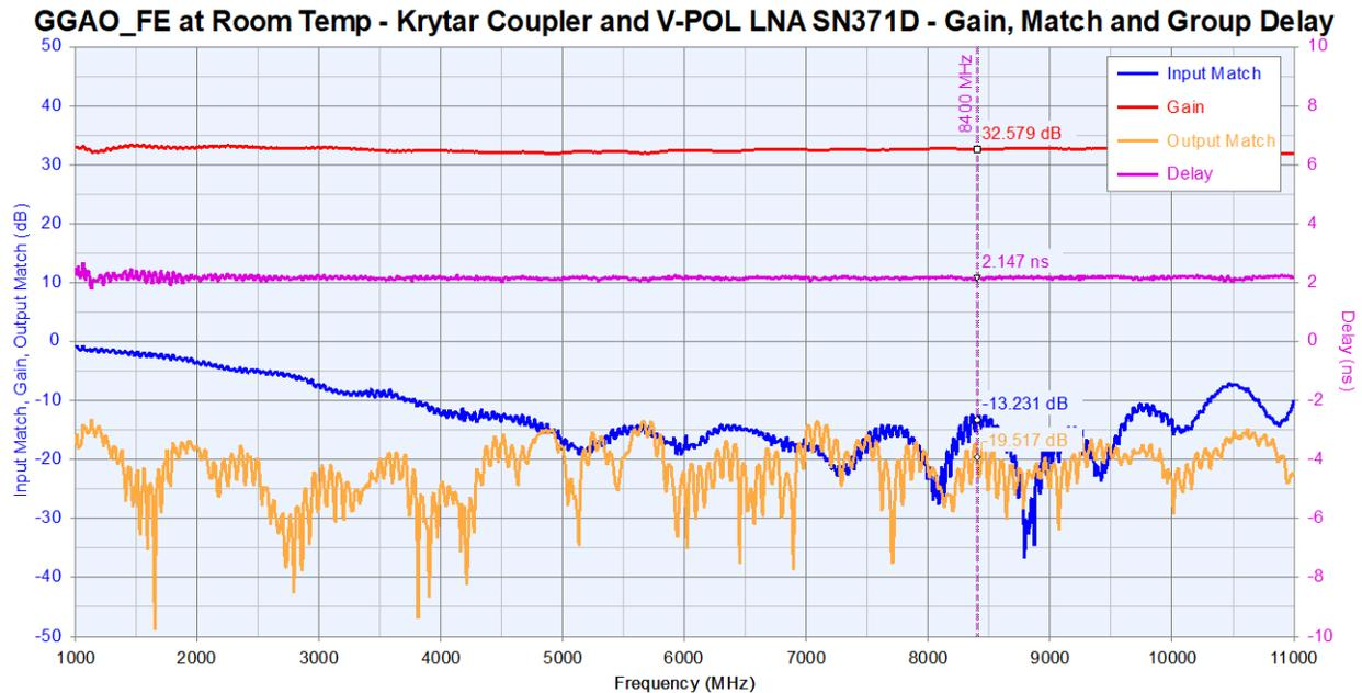
**Figure 7:** Same as Figure 6 but here for the V-polarization channel.
