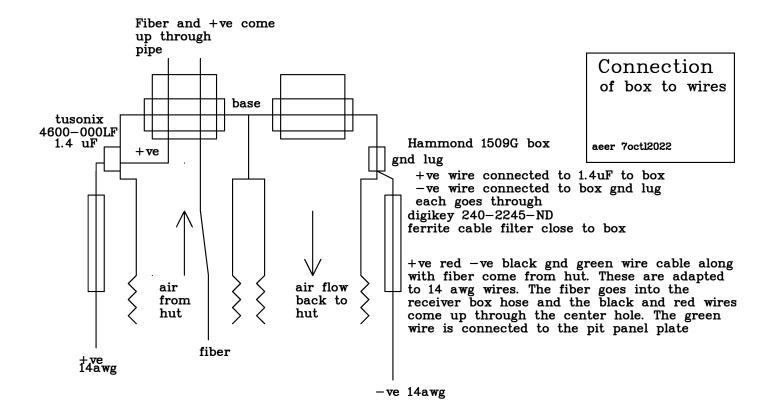
Figure 1. Diagram of the air flow and cable connections for the installation of EDGES-3 at the MRO.
