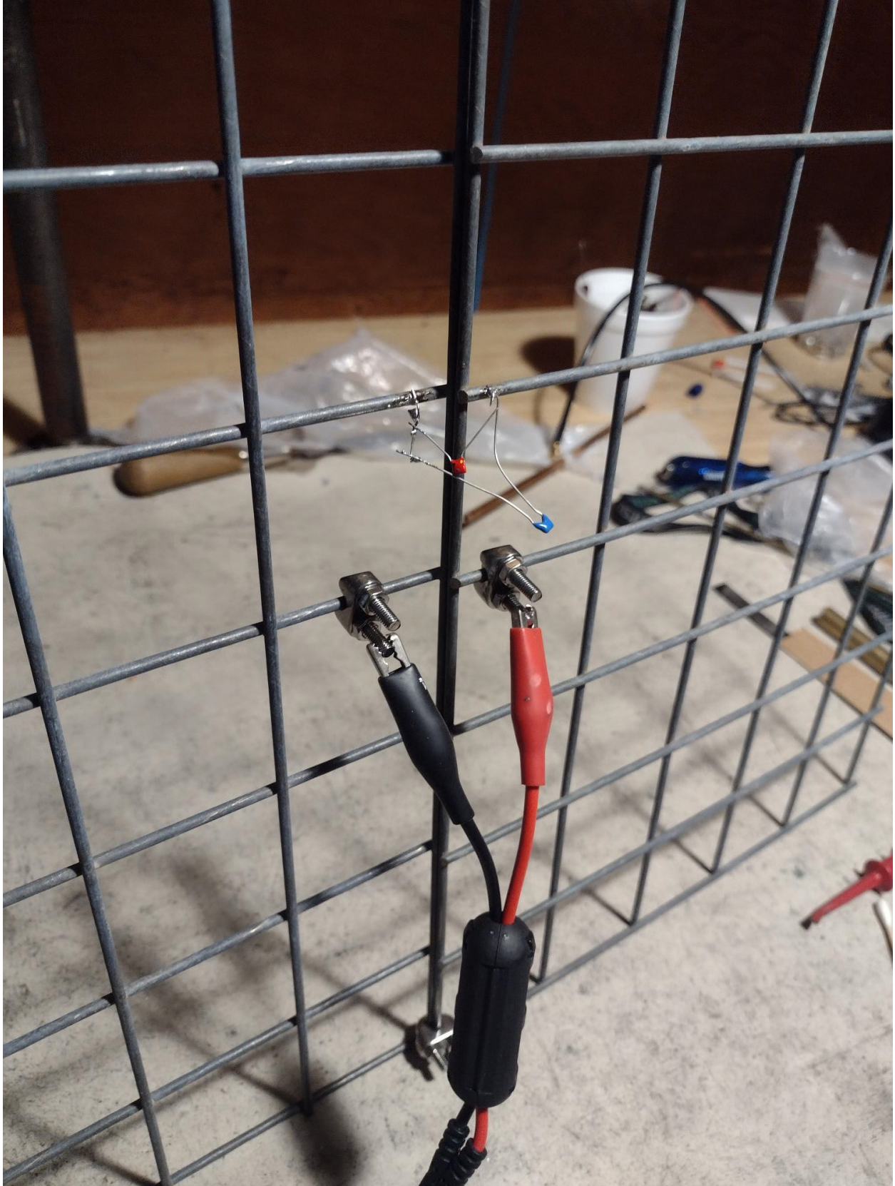
Figure 4. Photo of connections to mesh using crocodile clips
