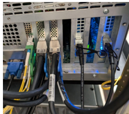
Figure: Back of Mark6 - 100GbE fiber in yellow
