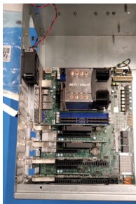
(a) Updated Mark6 interior with AMD EPYC, Supermicro H12SSL motherboard
