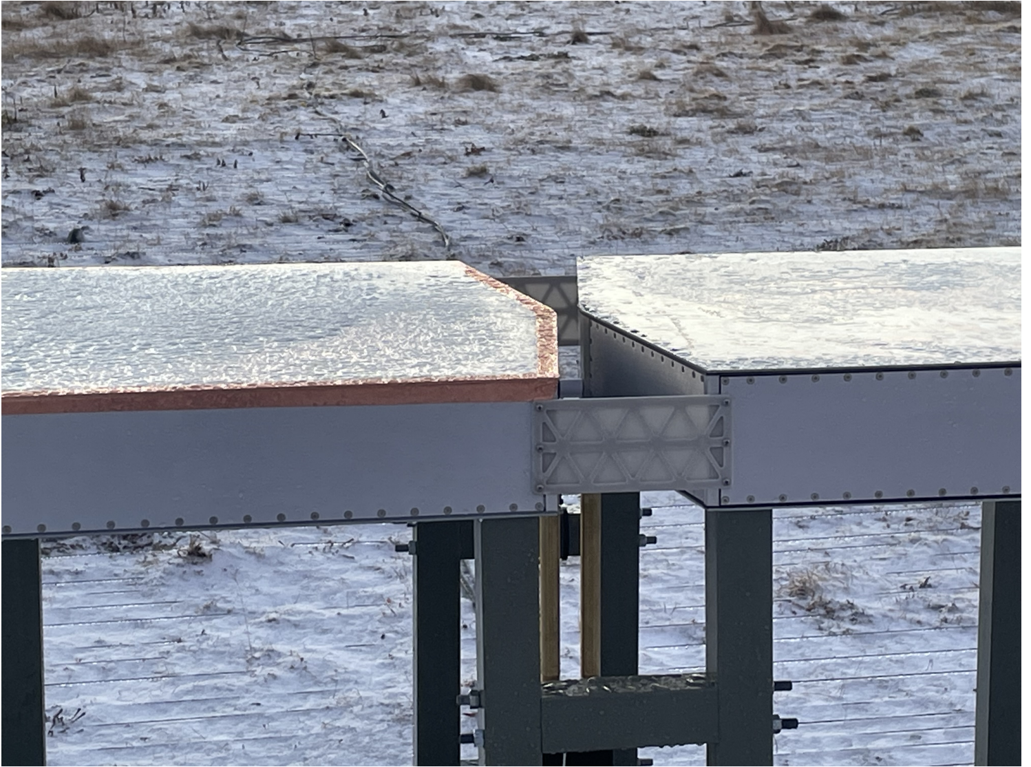
Figure 8: The surface of the antenna after the first night of observations. Ice had accumulated on the panels overnight, but melted away within a few hours of sunrise.
