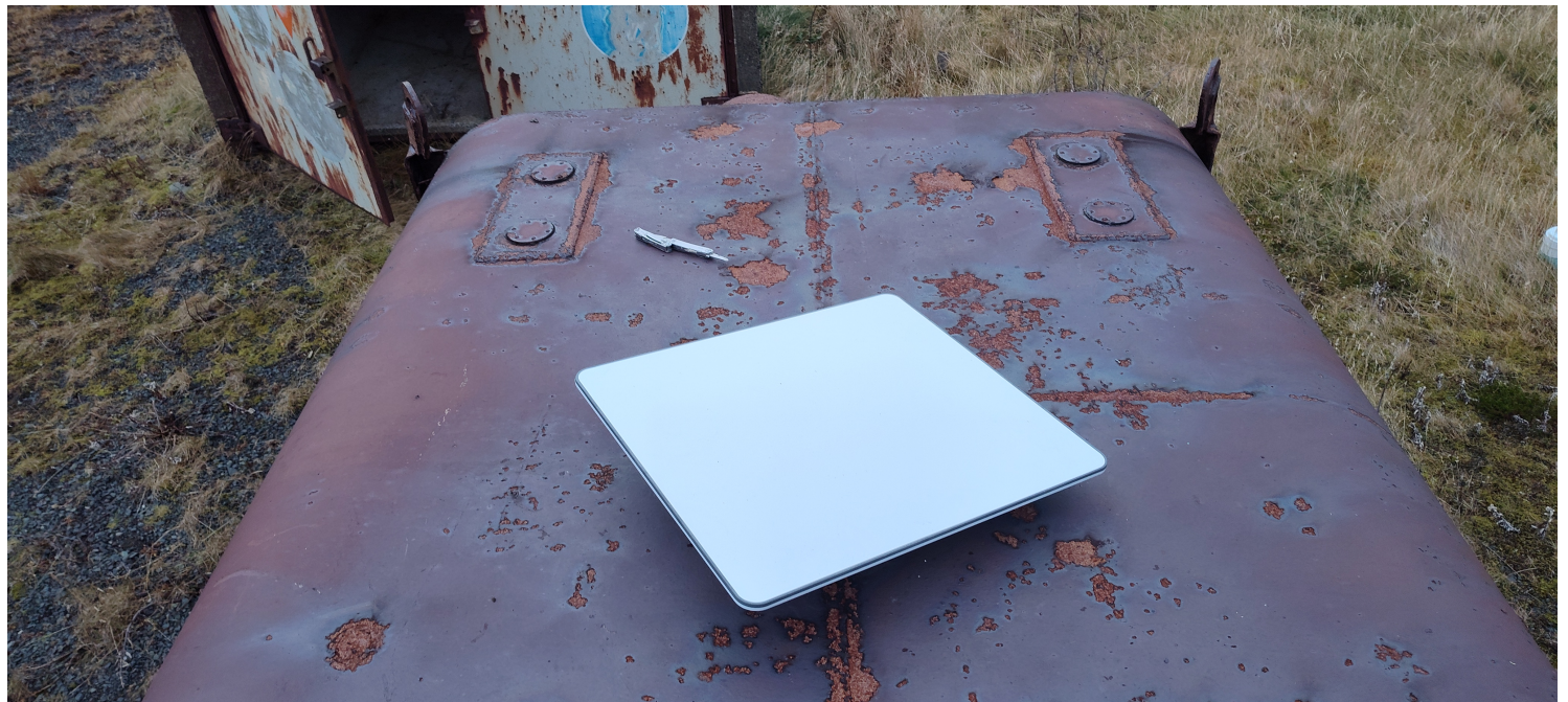
Figure 5: The flat high-performance Starlink antenna after installation on the hut roof. The antenna is oriented to face south, as that is the direction of the highest satellite concentration.
