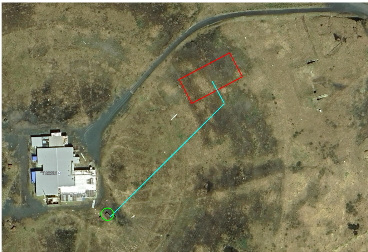
Figure 1: A satellite view of the EDGES-3 deployment site on Adak Island, AK. The red rectangle denotes the outline of the ground plane, the green circle is centered on the power/communications hut, and the cyan line represents the path of the power cable and fiber from the hut to the antenna. Vertical corresponds to north.
