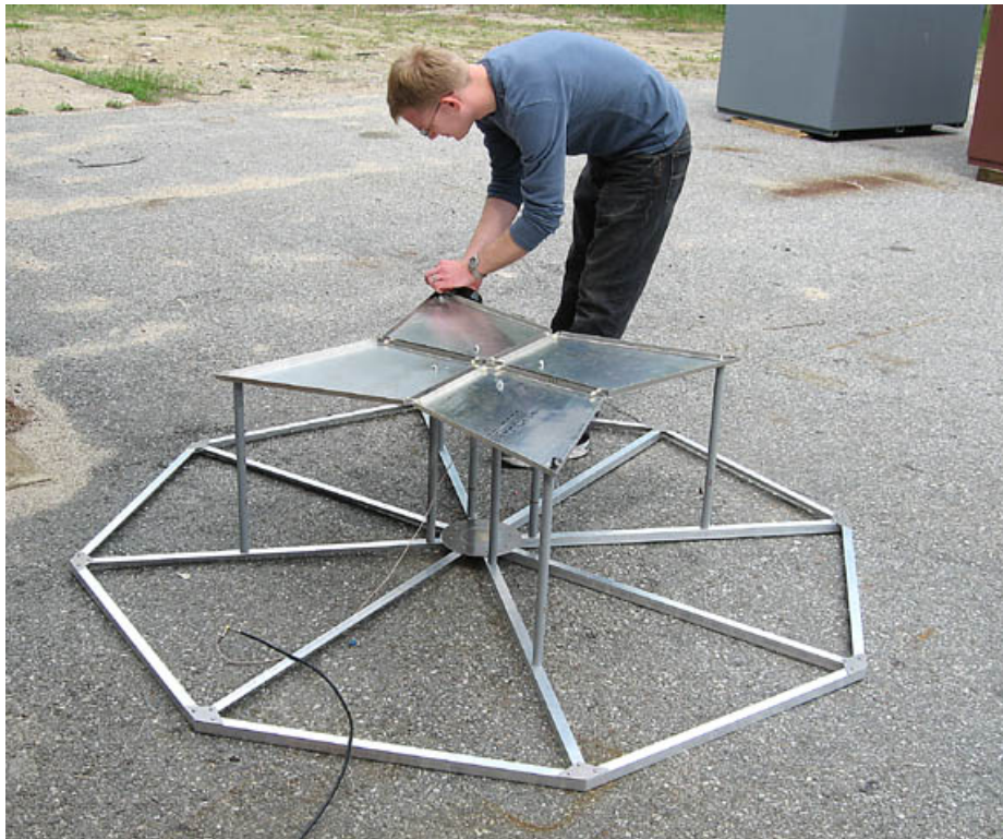
Figure 1 – Four-point dipole antenna during testing; shown while adding the 6-inch wire extensions to the tips of the dipole elements.
