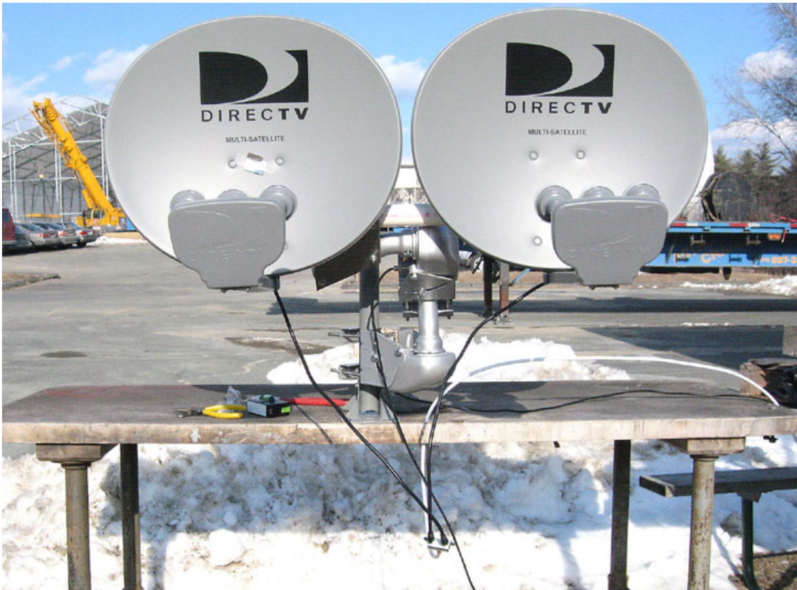
Figure 3. Front view of pair of dishes acting as a short baseline interferometer.
