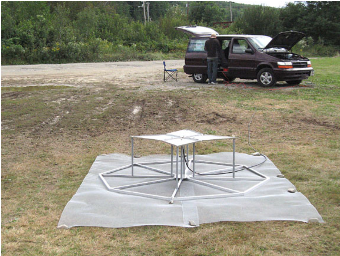
Figure 1. EDGES antenna at West Forks, Maine
