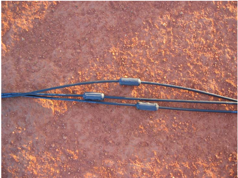
Figure 6. Ferrite common mode suppression filters used on cables in “EoR step” mode.
