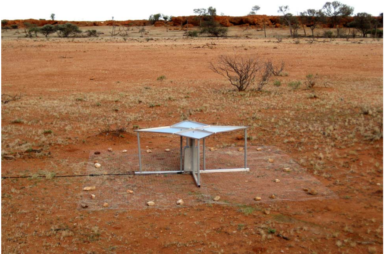
Figure 3. Operational configuration of the EDGES antenna, ground screen, and analog electronics enclosure.
