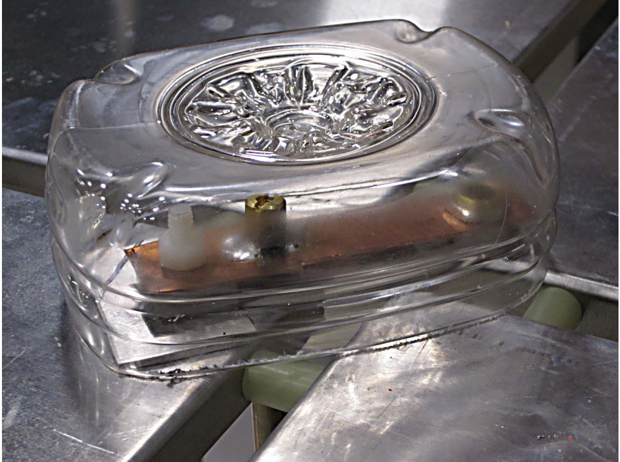
Figure 5. PET rain cover for top plate.
