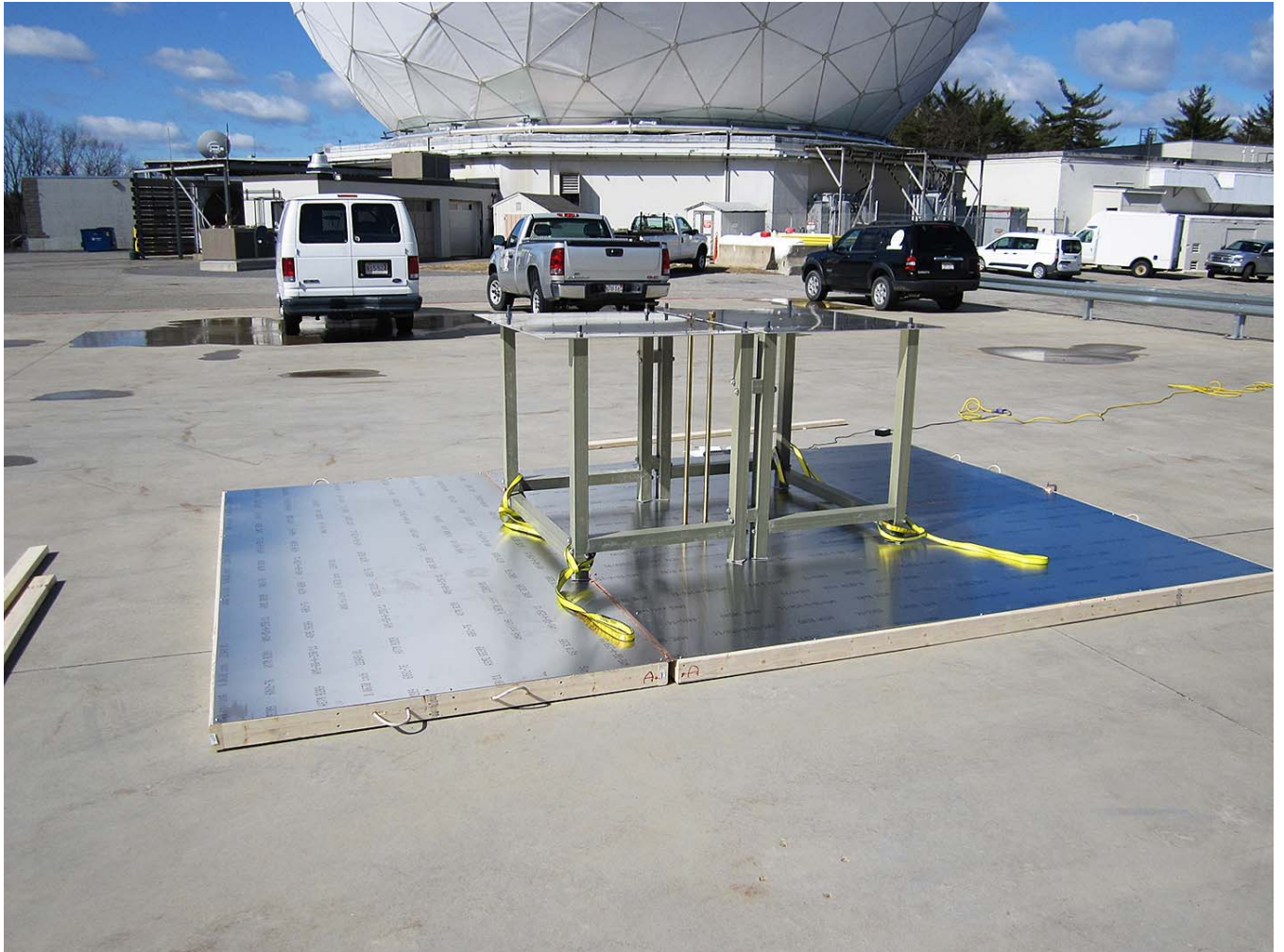
Figure 1. Low band (50 to 100 MHz) on temporary ground plane
