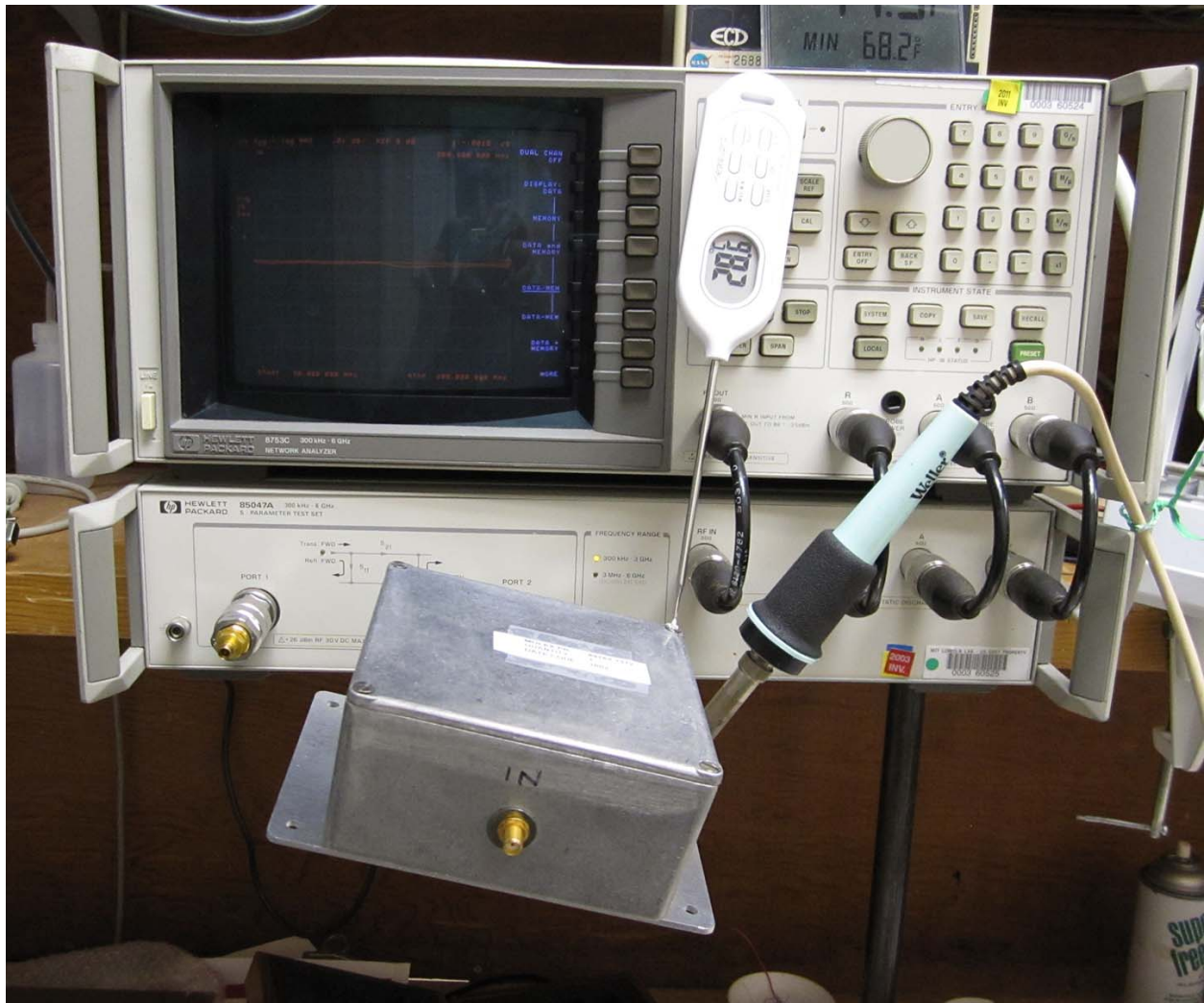
Figure 3. Cable attached to VNA port.
