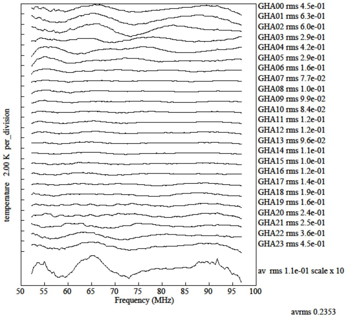
Figure 1a. Residuals to 5-term physical functions with beam correction using  $\epsilon=2.0$   $\sigma=2e-2$
