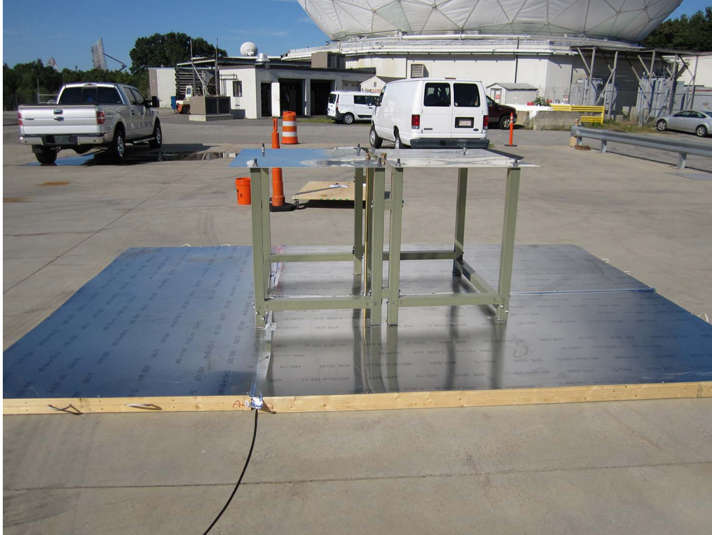
Figure 1. Second low band antenna under test at Haystack.
