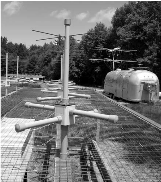
Figure 3. Close-up view of the deuterium array dipoles showing the directors that have been added to reduce the horizon response. Twelve Yagis of the RFI monitor and one set of active antennas pointed at zenith are mounted on the trailer in the background.
